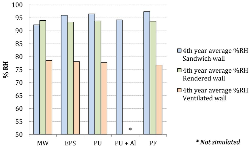
Figure 7. The yearly average relative humidity values for the exterior boundary of the thermal insulation layer during the first (top) and fourth year of the simulation period for the three studied wall structures given in Figure 1.
